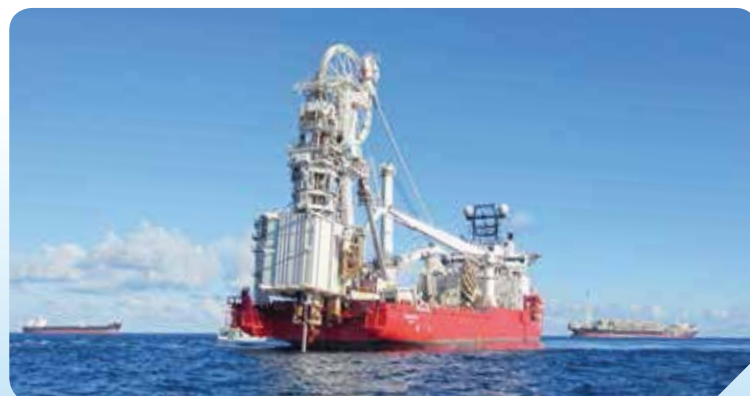
Seven Oceans J-laying BuBi  corrosion-resistant pipe on the Guar-Lula NE project, Brazil
